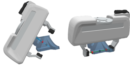
Figure 1: 6-DoF grasping based on left: surface normal and vertex or right: contact points.
