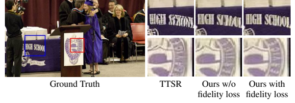
Figure 9. Ablation experiment on the fidelity loss. With the fidelity loss, we can obtain higher-fidelity reconstruction results.
